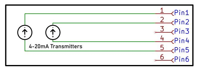
Voltage Should be Chosen to Suit 4-20mA Transmitters (12V In This Example)
