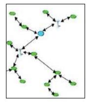
to transmit information from multiple points back to a central location. It is well suited for areas where each unit does not have a clear line of sight to a central point.
