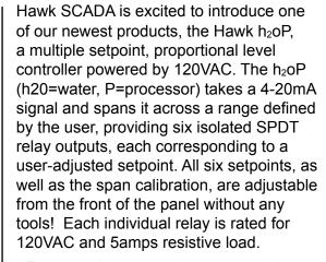
Each individual setpoint output can be configured as rising or falling (i.e. -- does this output need to be ON when the level is above or below the setpoint). This makes the unit capable of running a drain or a fill process such as: Wastewater: configure it to drain a wetwell; Groundwater: configure it to fill a tank.
